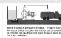
将液体A由膜送到B的方法可以照此法 This method can be adopted when sending the liquid from vessel A to vessel B
