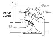
Drip-Tight Closing: Closure is obtained by directing line pressure or equivalent independent pressure into the upper chamber. This pressure on the large diaphragm area causes the valve disc to seal against the seat. (Ratio of diaphragm to disc area is 1.3 or greater.)
