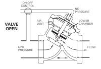
Full Open Operation: When closing pressure in upper chamber is relieved by venting the pilot line, the valve opens, positively, by line pressure on the disc
