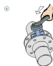
6. 待焊口冷却后再安装阀门。保证阀板有一定的开度 ( Stay cool joint before installation to ensure that the valve plate has the opening of the valve)
