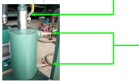
13, Checking the two pressure meter, if the pressure too high, please clean the first filter
