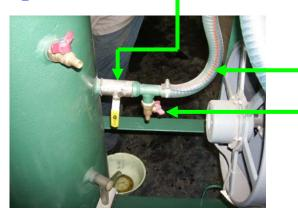
11, checking the liquid meter is the water is full close valve B and open the valve A, let the water out
