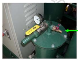
10, If here are oil in the pipe C, you can close the valve B and open the valve A let the oil back to vacuum separation tank
