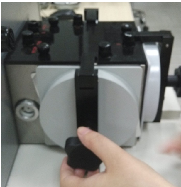
d. 盖上透气室盖，紧固密封
