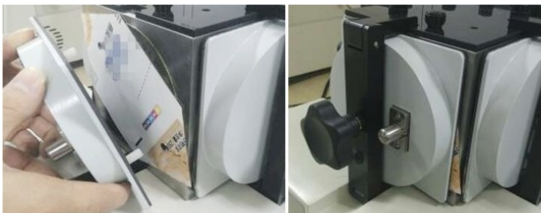
d. 盖上透气室盖，紧固密封
